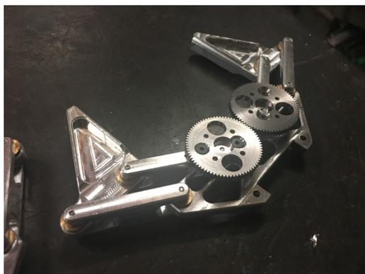
*Gripper machined assembly*
