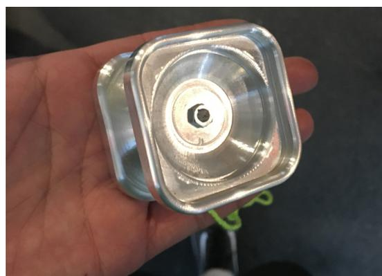
*The First Prototype was made on MITERS CNC mill and manual Bridgeport*
